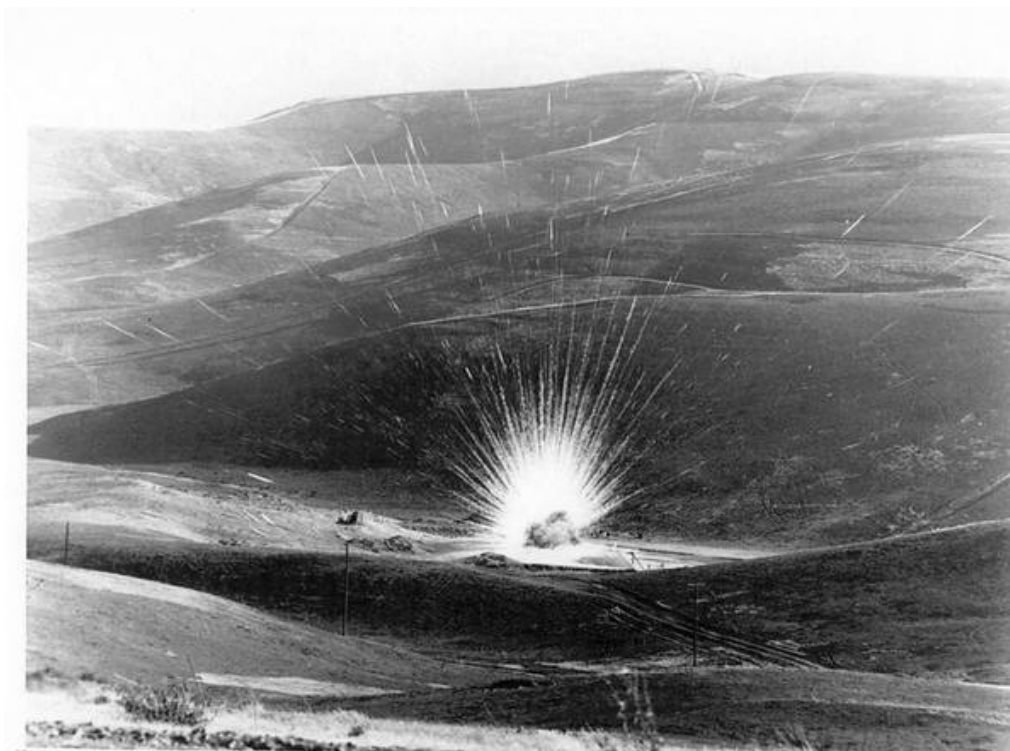
Hydrodynamic (bomb core) test on a firing table at Site 300, 1961. The bright "streaking" effect in the photo is likely from shards of pyrophoric metal, such as Uranium 238, hurtling through the air. U-238 is one of the contaminants of concern in the Site 300 Superfund cleanup. Photo: LLNL
